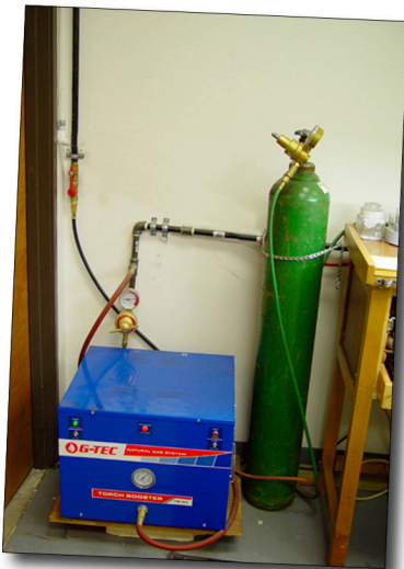
Torch Boosters can be installed next to jewelers' benches - they are quiet and do not require ventilation or other special site preparation
