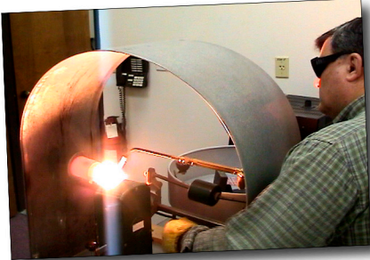
High-pressure natural gas easily melts platinum and improves the quality of platinum casting
