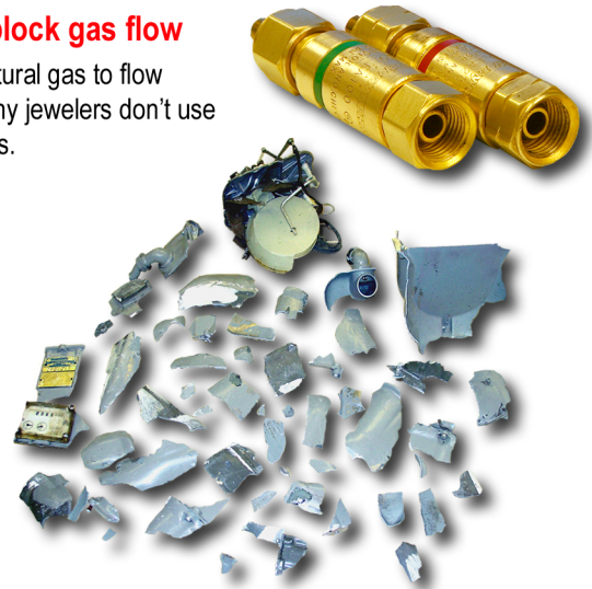
This is a gas meter which was destroyed in a flashback explosion at a New York City jeweler.
