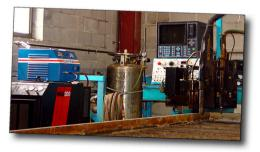
In Torch Booster mode DM-60 directly supplies torches cutting tables and manifolds with high-pressure natural gas.
