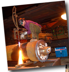
Cutting Thick Steel
