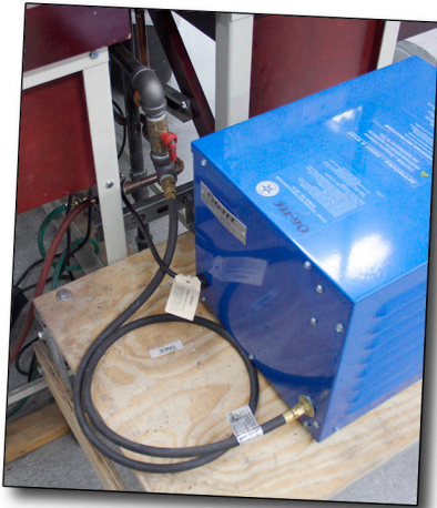
G-TEC supplies a flexible hose to connect your Torch Booster to the utility gas pipeline.
