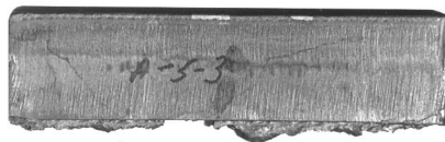
Cuts made with acetylene on 2" plate leave slag and need plenty of grinding
