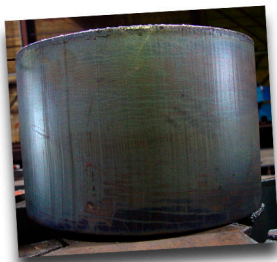
High-pressure natural gas makes high-quality cuts in the thickest steel
