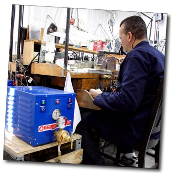
TB-15 / TB-30 Torch Boosters replace acetylene, propane and other fuel gases in cylinders and provide a steady supply of high pressure natural gas, up to 25 psi, directly from your standard utility gas line.
