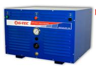
Refueler 180 - fills cylinders at a rate of 3 cf/min to 275 psi. Cabinet is 28"W x 20"D x 20"T, weighs 175 lbs. and uses 120V/60 Hz or 230V/50Hz 20 amp electric power.
