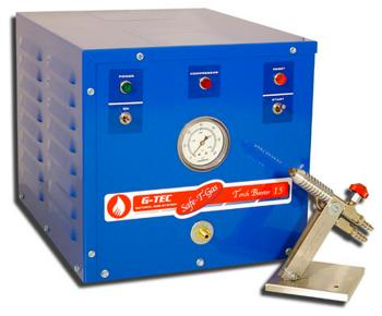
**A G-TEC Natural Gas Pressure Booster System** connects to your building's utility natural gas line then boosts the pressure to 5 psi for high-performance lampwork. Utility gas pressure is typically only 1/4 psi, which gives a weaker flame and poorer performance.
