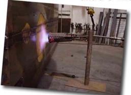
When you need high volumes of gas for pre-weld heating a G-TEC Torch Booster eliminates cylinder valve icing problems and never runs out - no empty cylinders to change
