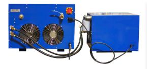
TB-250H Torch Boosters have a Compressor Module and a Cooler Module joined by 5' flexible tubing for installation flexibility. Both units operate from a single set of controls on the front of the Compressor Module. The Cooler Module can be stacked on top of the Compressor to reduce footprint space.
