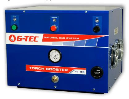
TB-60 / TB-125 Torch Boosters replace acetylene, propane and other fuel gases in cylinders and provide a steady supply of 25 psi natural gas directly from your standard utility gas line.
